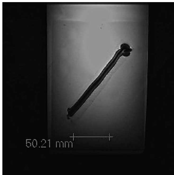
Figure 4. Artifact observed on MRI using a gradient echo pulse sequence. Note that the signal loss extended a maximum of 7 mm relative to the lead fragment.
